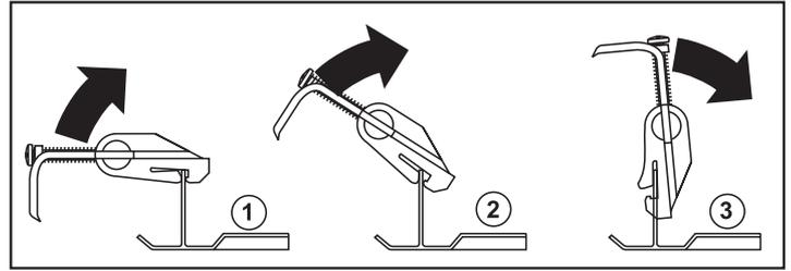
7. Turn the sink upside down and lay the worktop over the sink. Swing the clip into position. (This is the most effective method although if the worktop has been fixed to the cabinet, the sink can be placed in the aperture and the fixing effected from underneath).
